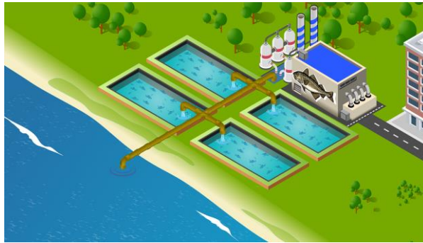
Figure 1.2. Land-based aquaculture facility equipped with extraction pumps to transport seawater into production units.
